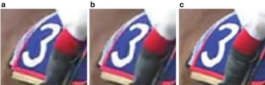
**Fig. 7.25** Subjective quality comparison of *RaceHorses* test sequence, POC = 20, QP = 32, LP condition: (a) SAO is disabled, (b) SAO is enabled, (c) original (uncoded) sequence
