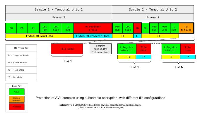
Figure 1 Subsample-based AV1 encryption.
